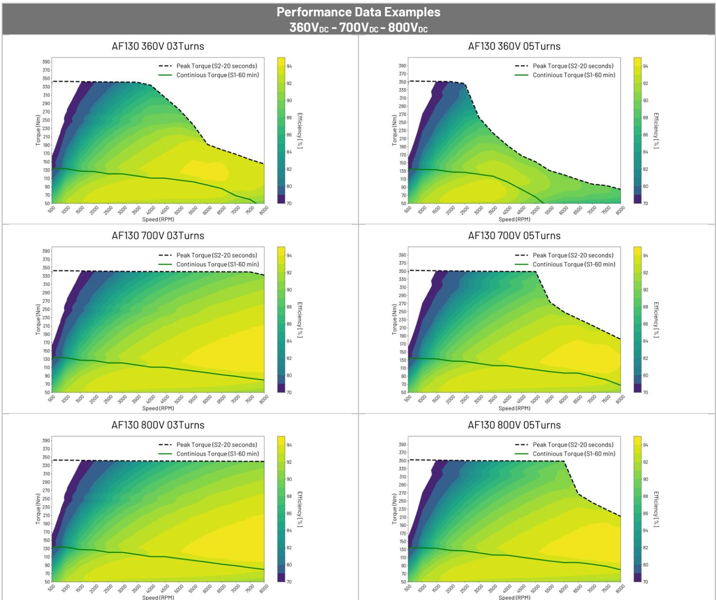
All values in the graphs are quoted for 45°C ambient with coolant at 55°C inlet temperature and 8 LPM flow rate. Efficiency will vary based on Voltages and Turn count.
