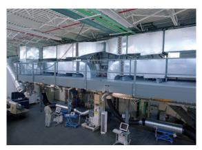
Figure 2. Laboratory setup for RTU performance characterization at NREL
