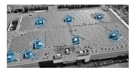
In 2019, a leading Big Box Retailer implemented the Turntide Smart Motor System™, a simple, drop-in energy conservation measure that reduces HVAC energy use in rooftop units (RTUs) found in its store locations. Turntide moved from a successful pilot to a phase 1 rollout across over 300 stores.
