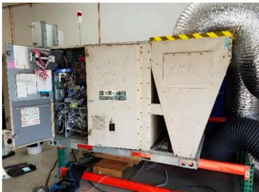
**Figure 1. Laboratory setup for fan performance characterization**
